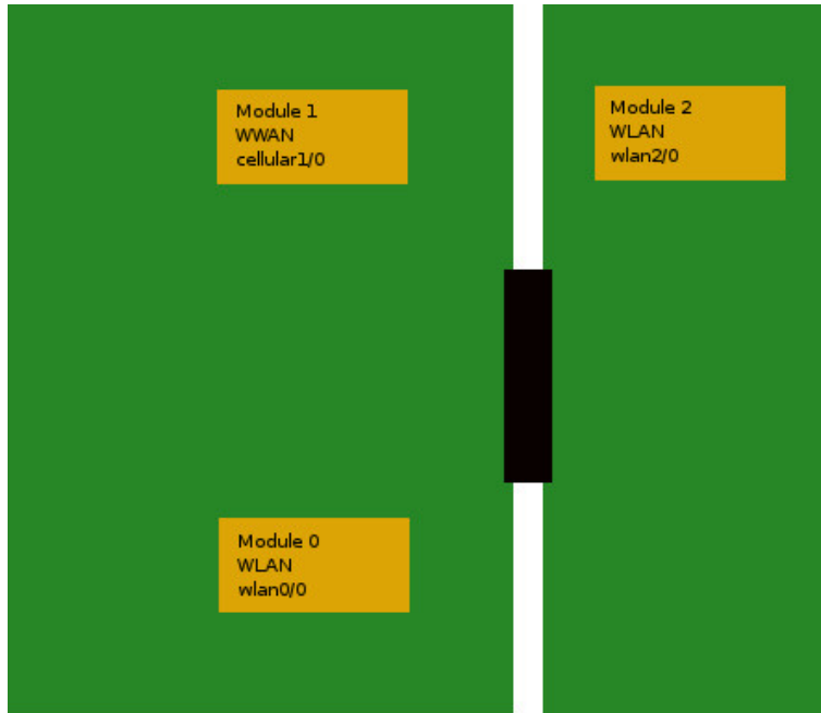
Fig. 21: Option 1, with two WiFi modules
