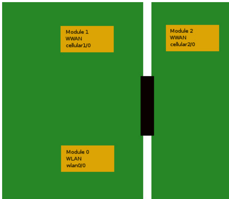
Fig. 22: Option 2, with one, two or no cellular modules
