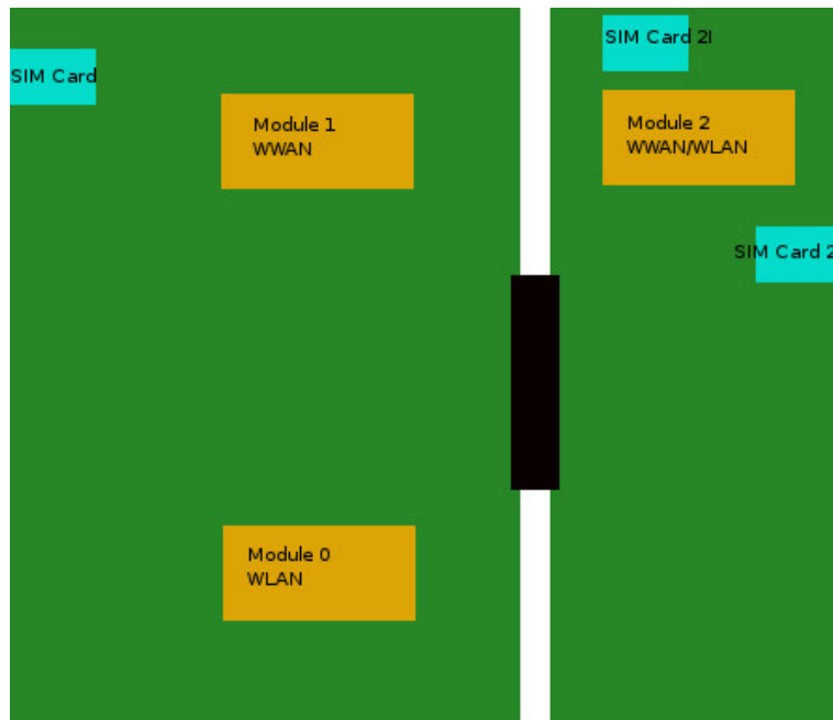
Fig. 18: SIM Card 21 and SIM Card 2 for Module 2, SIM Card for Module 1
